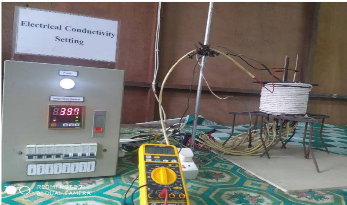
**Figure-4** Temperature dependent electrical resistances measurement
